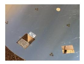
Step 6: Secure the Primary Pilot Burner Media Cage to the Flat Burner Pan as shown in the photo at right.
