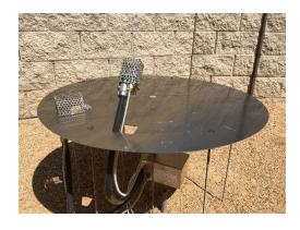
Step 8: Secure the Secondary Pilot Burner to the Flat Burner Pan as shown in the photo at right.
